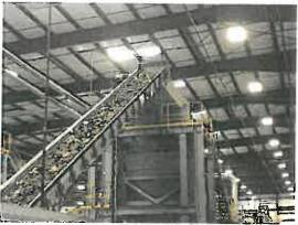
Post-Shredded MSW Moving into the Processing System
