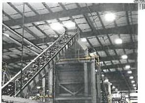
Post-Shredded MSW Moving Into the Processing System
